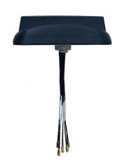
Gar multi-port vehicle antennas provide an excellent solution for Public Safety, Transportation and Aftermarket Fleet applications. Configured for 2-port MIMO operation over the 3G / 4G / 5G / ISM / CBRS bands and 2-port MIMO operation over the low//high frequency Wi-Fi bands, with an additional 5th port for GNSS. Now with QMA connectors for rapid installation.
